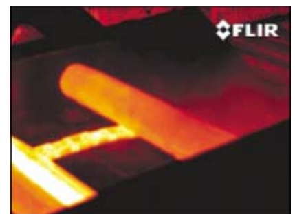
Below: The Thermovision infrared camera helps the operator see through the steam to safely complete his tasks.
