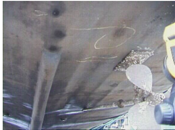
Figure 8. A common practice to extend the life of the bottom of a wooden boat is to sheath it in FRP. It is used to reduce maintenance and prevent marine organisms (e.g., Terado worms) from boring into the wood. Sometimes the physical bond between the wood and FRP breaks down, and water gets trapped in the interstitial space. The wood continues to decay and the FRP disbonds from the wood. Coolness in the infrared image shows the extent of water entrapment and disbonding that can be heard when sounding the hull with a percussion hammer.
