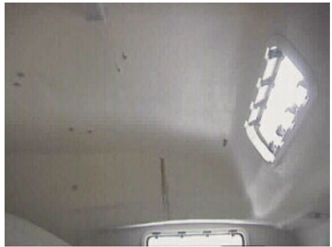
Figure 9. This is the interior ceiling of a FRP constructed catamaran sailboat. Brown fluid observed running out down the ceiling wall visually shows there is a problem with water intrusion. The ceiling is a sandwich construction composite of an outer skin of FRP, an intermediate core of wood, and an inner skin of FRP. The black and white pallet infrared image (left) shows the extent of moisture intrusion.
