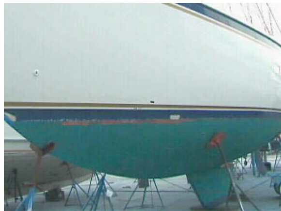
Figure 6. This is the side of a sailboat constructed with FRP. The sailboat sustained impact damage and there was a faint visual sign of delamination. The infrared image shows warmer temperatures, revealing the extent and pattern of delamination in the FRP.
