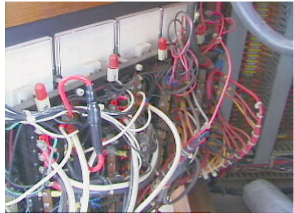
Figure 1. This is the back of an electric distribution panel in a 40-foot boat. Visual inspection shows that the wires are intact, wire insulation and terminals were free of burn or scorch marks. Infrared view shows that one of the wires in the bundle of wires is much hotter than the others. The heat and resistance in this wire caused its magnetic circuit breaker to trip intermittently.
