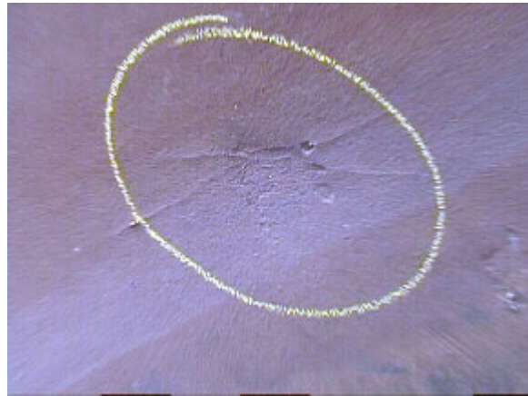
Figure 5. The area circled in yellow shows an unusual indentation in the hull of a boat constructed with FRP. Area visually appears dry. Infrared image shows cooler temperature, revealing moisture intrusion in this portion of the hull.
