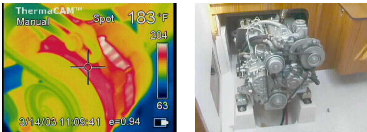
Figure 4. Views of a 3-cylinder naturally aspirating diesel engine. Visual photograph (right) shows the engine with a factory installed low amperage output 12VDC alternator. Owner replaced original “wet cell” battery bank to one with a larger capacity. The new battery bank was much too large to be effectively charged by the factory installed alternator. There were no visual signs that the alternator was being overworked, however the battery bank would never get fully charged and batteries suffered from sulfation. Infrared showed windings in alternator were hotter than expected. This visual evidence coupled with measuring low input voltage at the battery terminals solidified the recommendation why the buyer should upgrade to a higher amperage output alternator.
